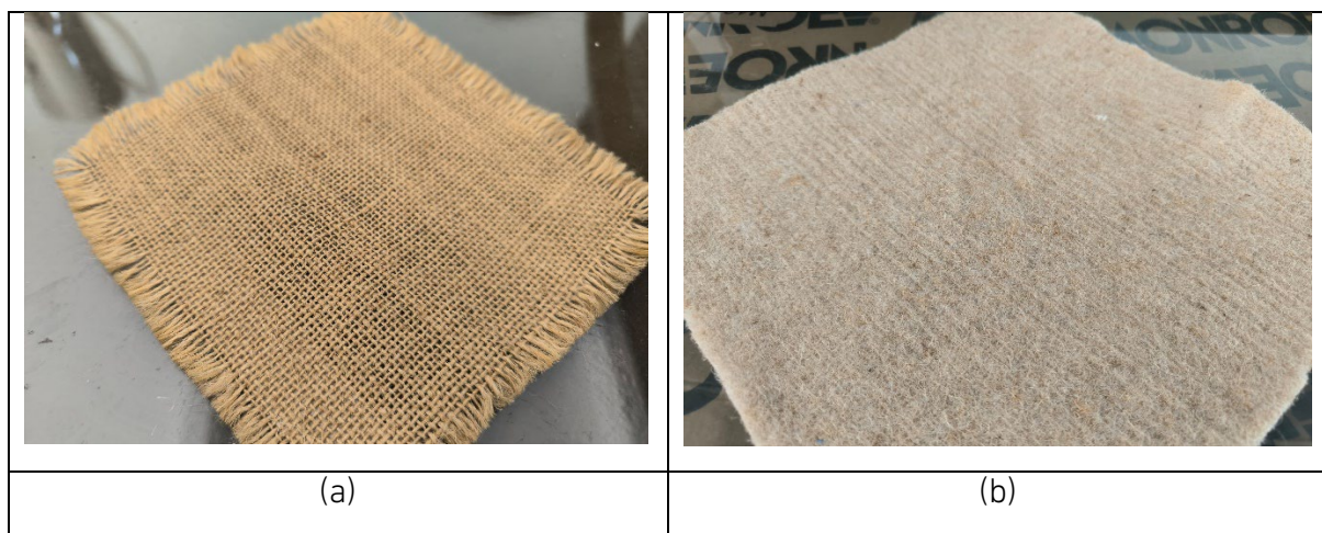
Figure 3.1. Natural Fibre Samples Used in the Study (a) Jute Woven Mat, and (b) Kenaf Non-woven Mat
