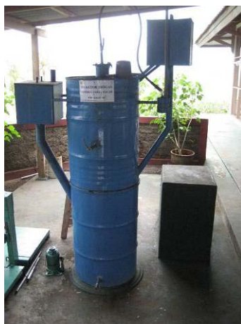
Biogas reactor from Jatropha residue
