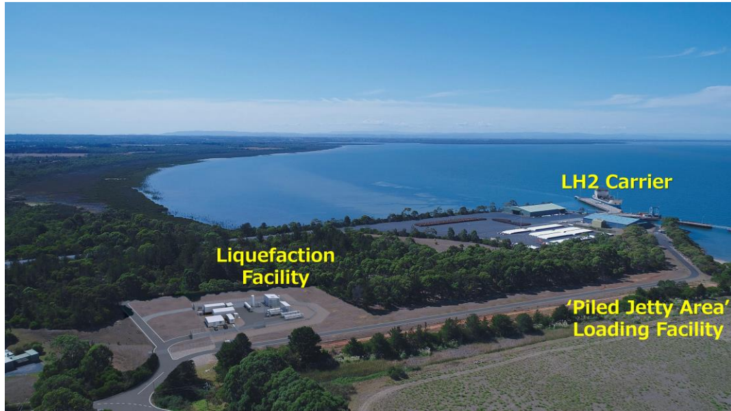
Figure 4.10: Hydrogen Liquefaction/Loading Facility (Hastings/Image CG Diagram)
