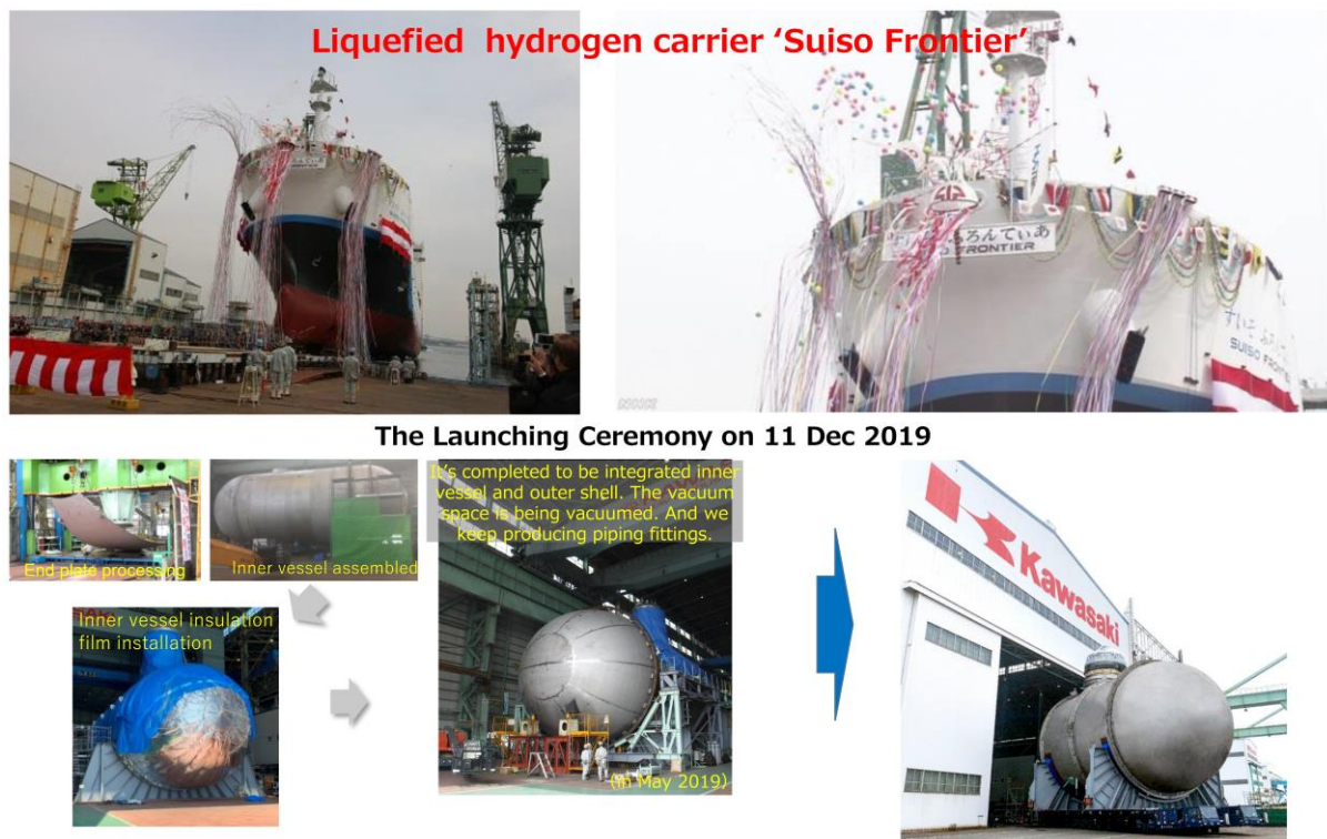
Figure 4.14: Pilot LH2 Carrier, Cargo Containment System Construction Status (Kawasaki Factory)
