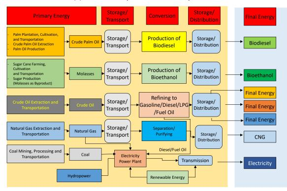
CNG = compressed natural gas, LPG = liquefied petroleum gas. Source: Pongthanaisawan (2012).
