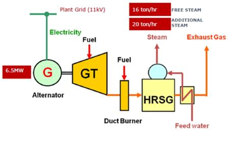
1 x GTG Output @ ISO Rating7800 kW1 x GTG Output @ 32° C (Gross)6540 kW1 x HRSG Unfired Steam Output (Gross)16.9tph
