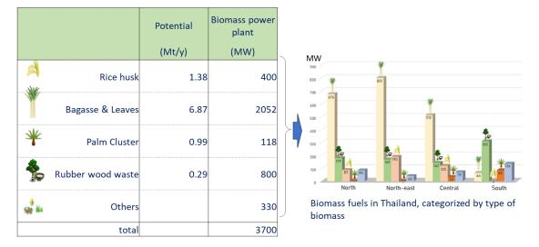
Figure 3.37. Biomass Potential and Current Biomass Power Plant
