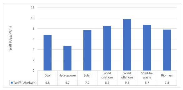
Figure 3.59. The Unit Cost of Electricity by Type of Generation in Viet Nam
