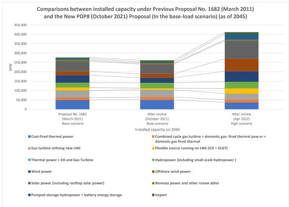
Figure 3.49. Installed Generation Capacity by Energy Source for PDP8 (as of 2045)
