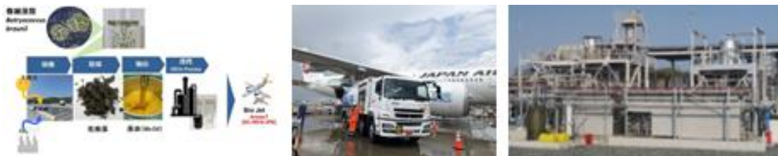
Figure 2.19. Biojet Fuel Process (Algae Photosynthesis, FT Synthesis)
