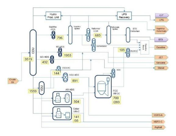
Figure 2.10. Refinery Equipment Configuration in Japan
