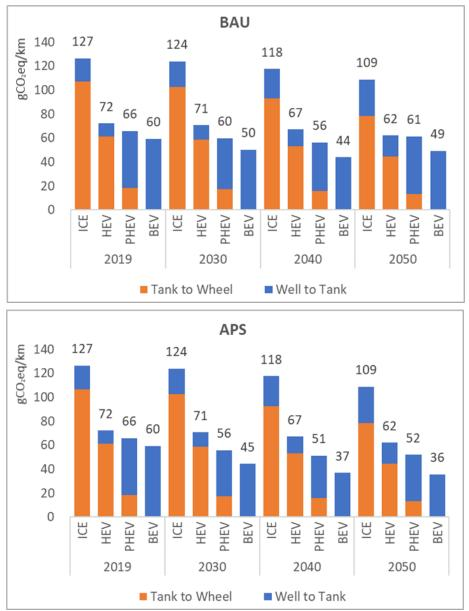
Figure 2.8. GHG Emissions based on Well-to-Wheel by Powertrain (Thailand)
