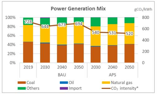
Figure 2.4. Power Generation Mix and CO<sub>2</sub> Intensity (Malaysia)
