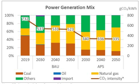
Figure 2.5. Power Generation Mix and CO<sub>2</sub> Intensity (Viet Nam)
