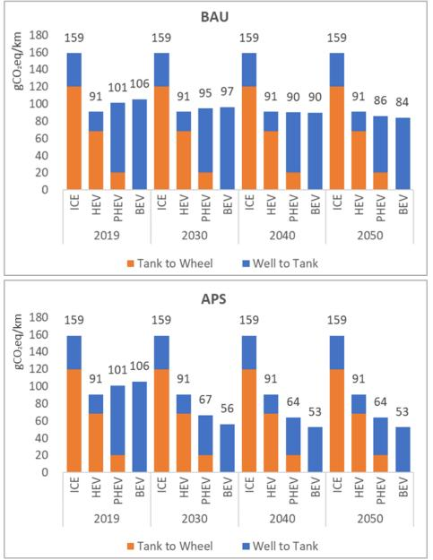
Figure 2.11. GHG Emissions based on Well-to-Wheel by Powertrain (Brunei Darussalam)
