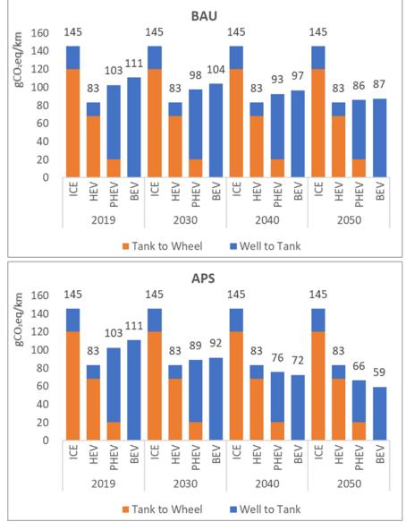
Figure 2.7. GHG Emissions based on Well-to-Wheel by Powertrain (Indonesia)
