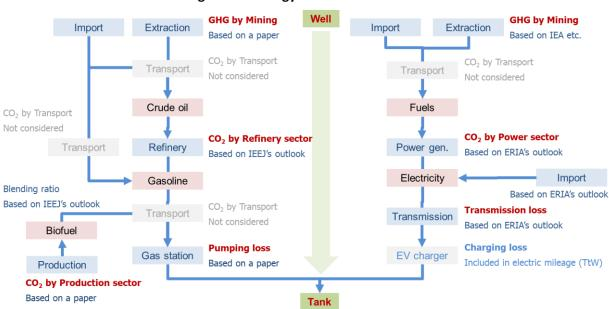
Figure 2.1. Energy Flow of Well-to-Tank
