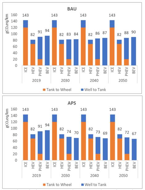
Figure 2.9. GHG Emissions based on Well-to-Wheel by Powertrain (Malaysia)
