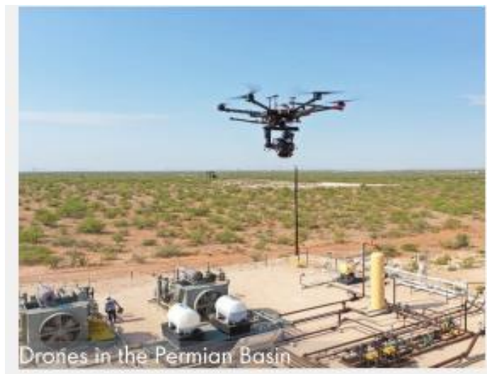
Figure 4.5. Shell's Methane Measurement Using a Drone in Permian Basin
