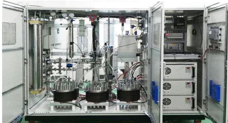
Figure 5.8. Equipment of 200 Nm 3 /h (1 MW) PEM (size: 2400*1700*2000)
