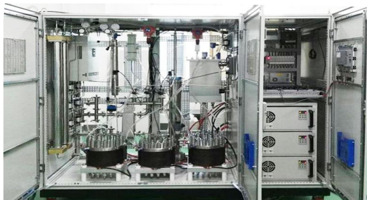
Figure 5.8. Equipment of 200 Nm 3 /h (1 MW) PEM (size: 2400*1700*2000)
