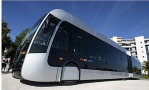
Eight 18 meter long Van Hool fuel cell buses operate 6 km express route.
