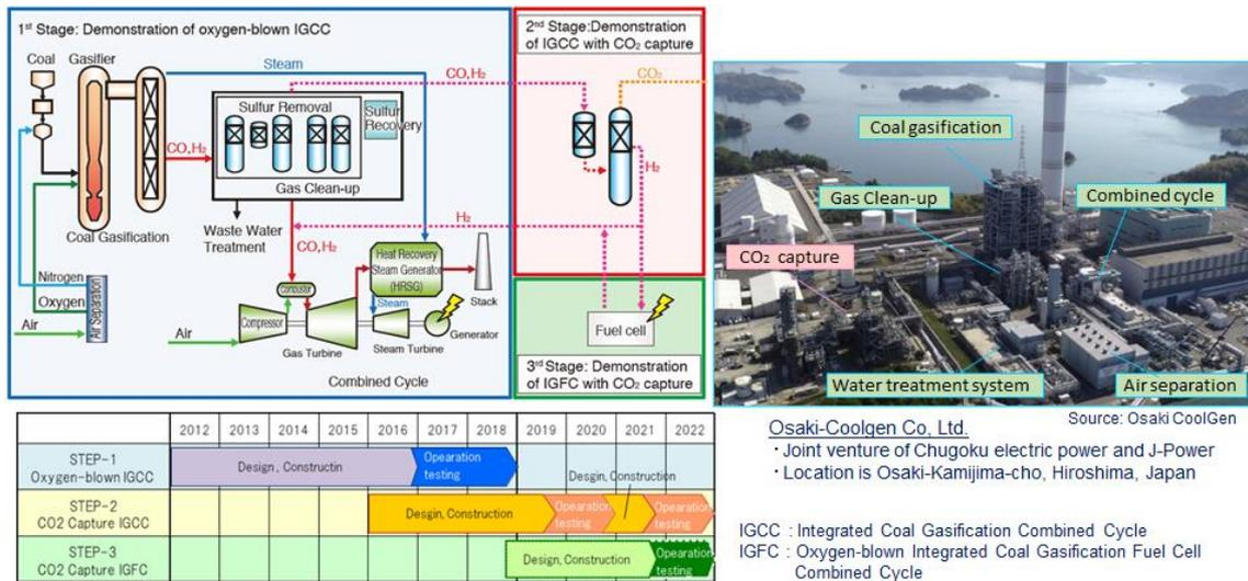
IGFC = integrated coal gasification combined cycle + fuel cell.
