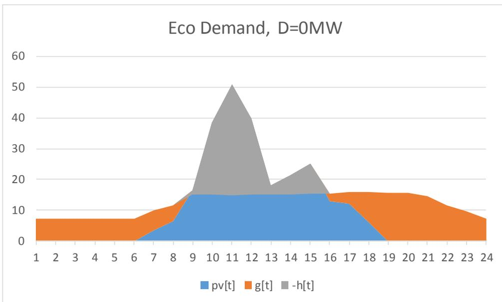
D = capacity of diesel generator, g = discharged electricity from the storage, -h = charged electricity in the storage, MW = megawatt, MWh = megawatt hour, p = generated electricity in diesel generator, PV = generated electricity in solar photovoltaic, t = time in hour.
