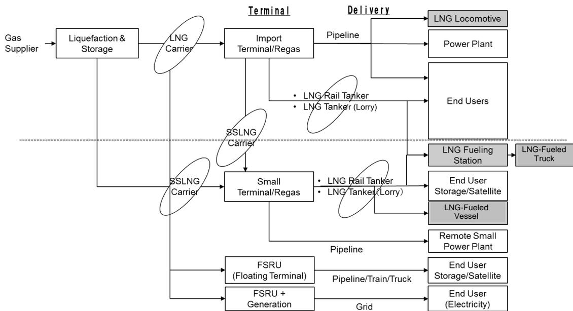
FSRU = floating storage and regasification units, LNG = liquefied petroleum gas, SSLNG = small-scale liquefied petroleum gas.
