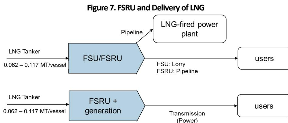
FSRU = floating storage and regasification unit, FSU = floating supply unit, MT = megatonne.
