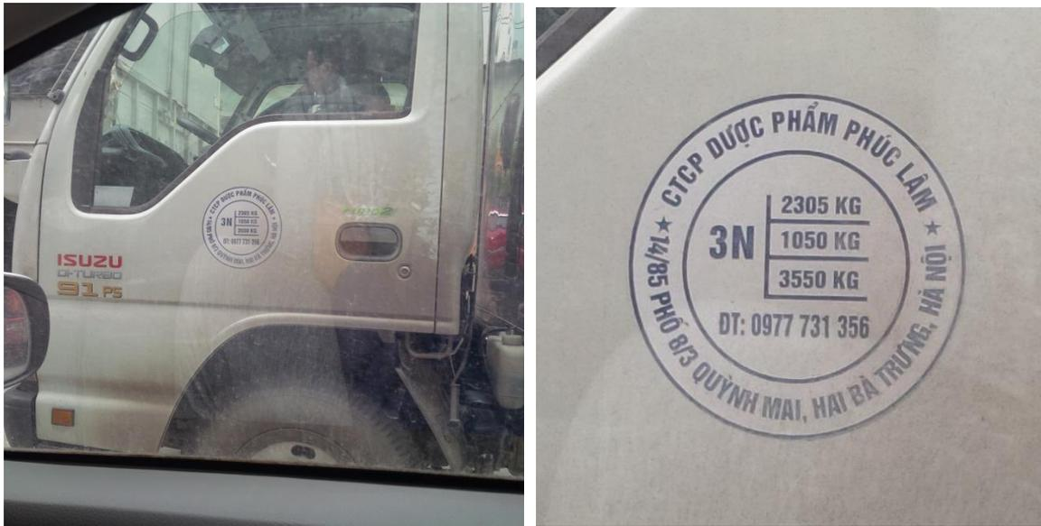
Note: These characters show the name of the company that owns the truck, the number of drivers and passengers allowed (maximum of three persons), the permitted loads for each axle, and the total weight of the vehicle.
