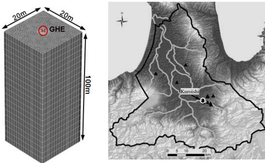
Notes: Single ground heat exchanger model (left) and locations of thermal response tests and single ground heat exchanger models (right).
