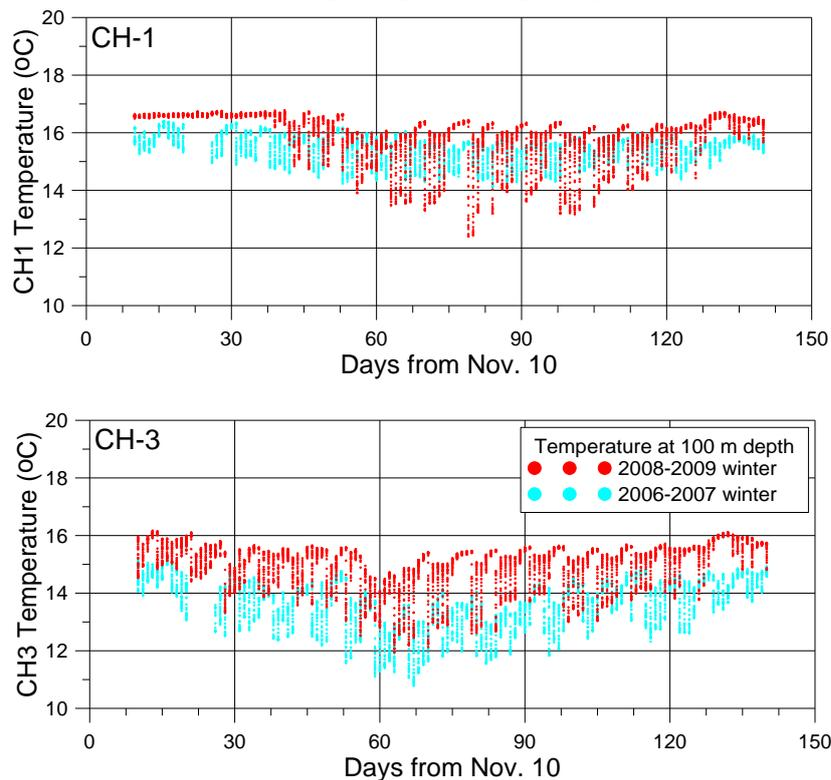
Note: CH-1 and CH-3 denotes the borehole heat exchangers (BHEs) at different locations.
