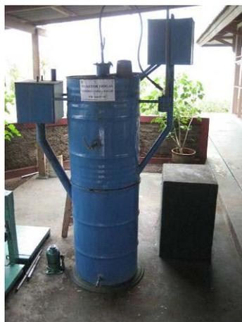
Biogas reactor from Jatropha residue
