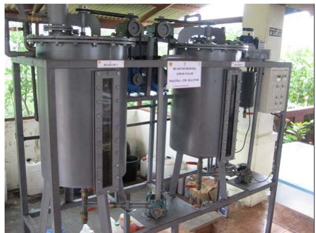
Biodiesel processing reactor
