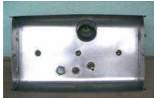
Fig.3.3.6 Results of Fuel Tank Test : Effects of Improving Oxidation Stability
