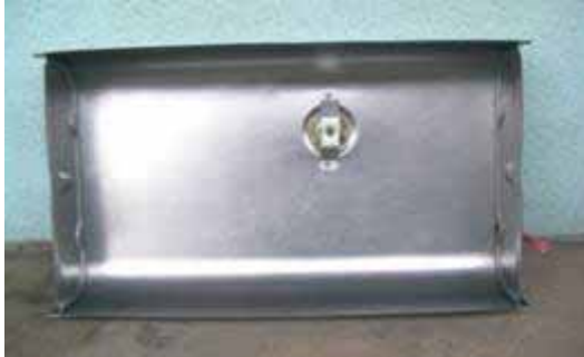
Fig.3.3.6 Results of Fuel Tank Test : Effects of Improving Oxidation Stability
