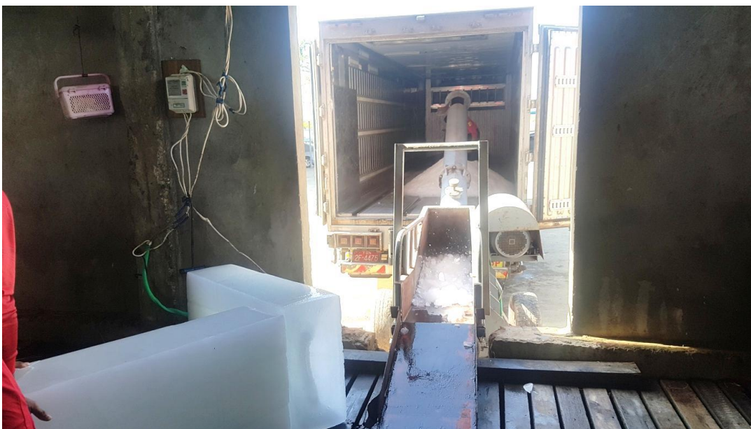
Figure 6.21: Loading Ice into a Refrigerated Truck from Company Owned Ice Plant
