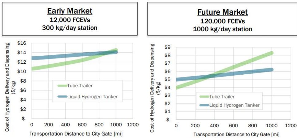
Figure 4.20 Example of Hydrogen Delivery Cost of CH 2 and LH 2 (US Department of Energy)
