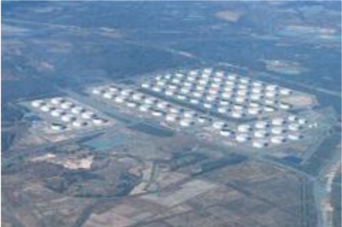
Figure 2-1. Typical Ground Stockpiling Facility
