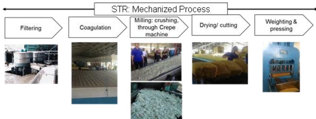
Figure 2-22: TSR processing process
