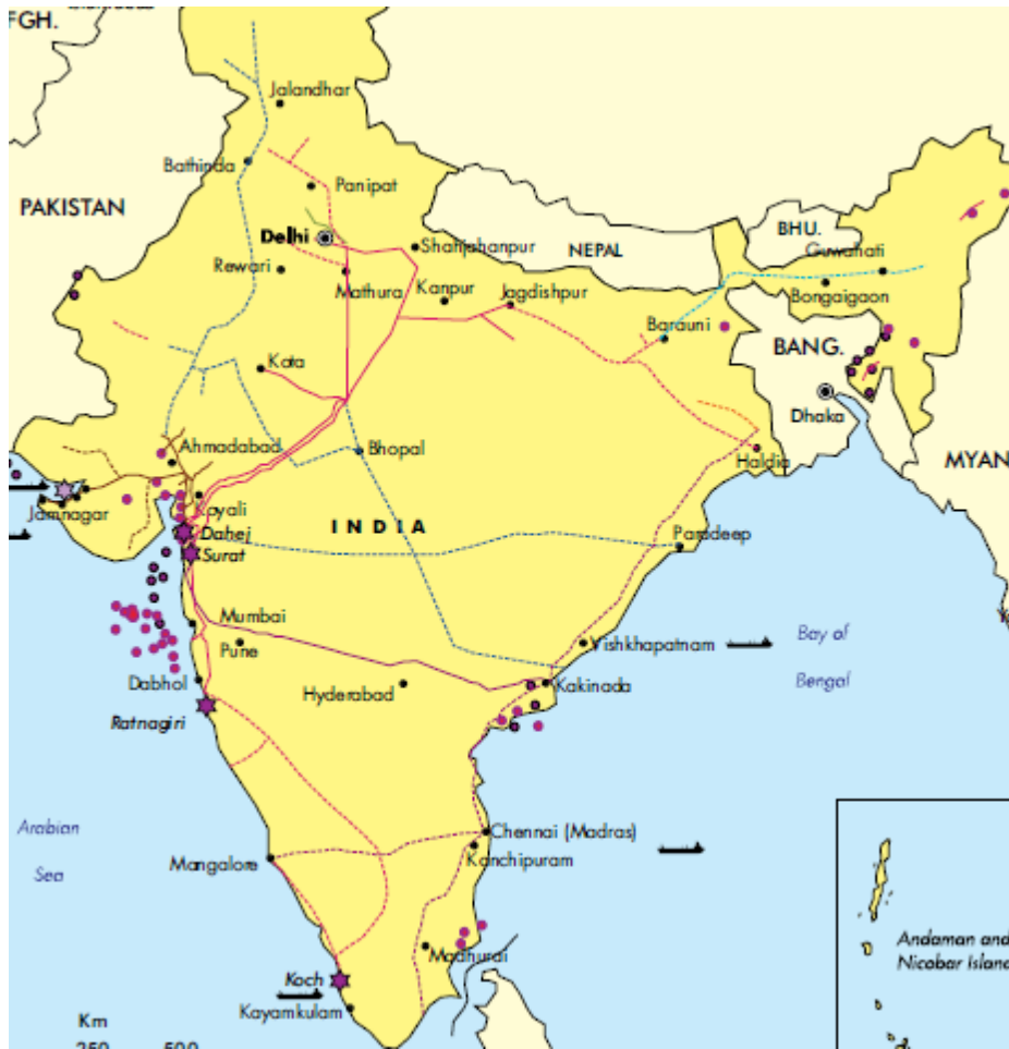
Figure 3.4: Natural Gas Pipeline Network in India
