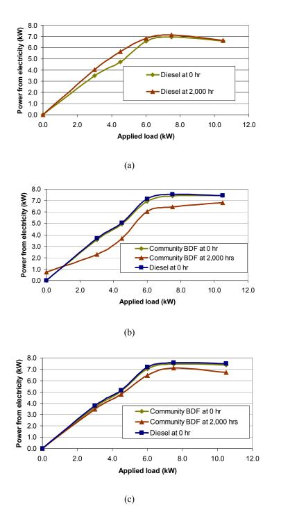
Figure 52 Performance test results of engine before and after running on (a) diesel: engine no. 1, (b) biodiesel: engine no. 2 and (c) biodiesel: engine no. 3 for 2,000 hrs
