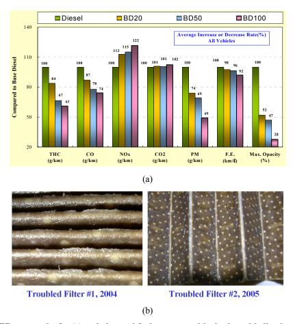
Figure 49 KIER test results for (a) emission and fuel economy with rice bran biodiesel, and (b) troubled fuel filter due to insufficient biodiesel quality
