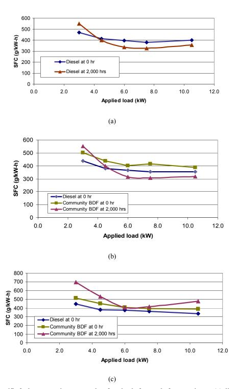
Figure 54 Specific fuel consumption test results of engine before and after running on (a) diesel: engine no. 1, (b) biodiesel: engine no. 2 and (c) biodiesel: engine no. 3 for 2,000 hrs
