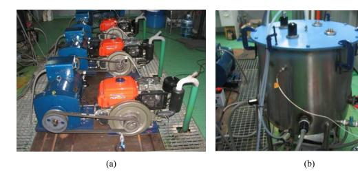
Figure 50 Experimental setup showing (a) Kubota engine coupled with electricity generator and (b) resistance heater coil
