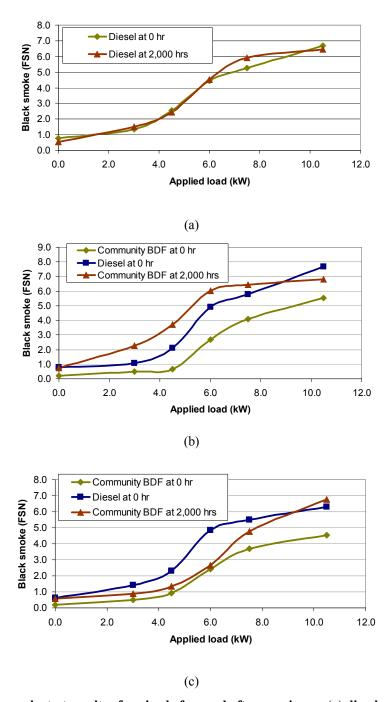
Figure 53 Black smoke test results of engine before and after running on (a) diesel: engine no. 1, (b) biodiesel: engine no. 2 and (c) biodiesel: engine no. 3 for 2,000 hrs
