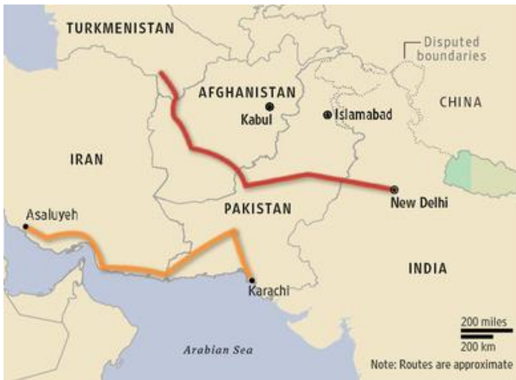
Figure 2.6: Pipeline Routes of IPI and TAPI Projects
