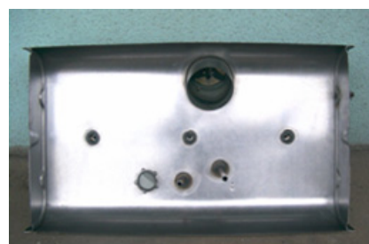
Figure 16 Effects of oxidation stability on fuel tank corrosion
